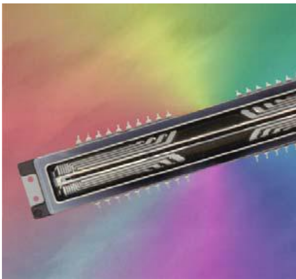
CCD trilineare Kodak KLI-14403, 3x14404 pixel
